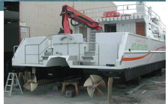
"Predator", a Richard McBride designed planning catamaran, was originally built by Rex Barnett of Barnett Engineering in Blenheim. Rex also performed the recent lengthening and propulsion refit. The twin hulls were modified slightly to suit the relatively simple mounting of the Q-SPD drives.
